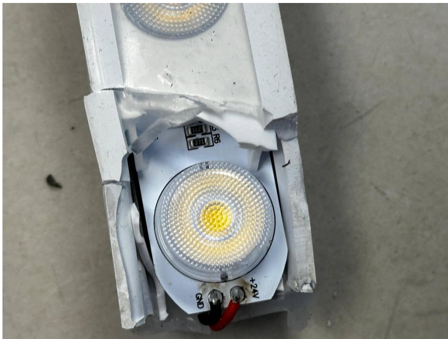
Photo 5: Test result of IP6X and IPX7 test
