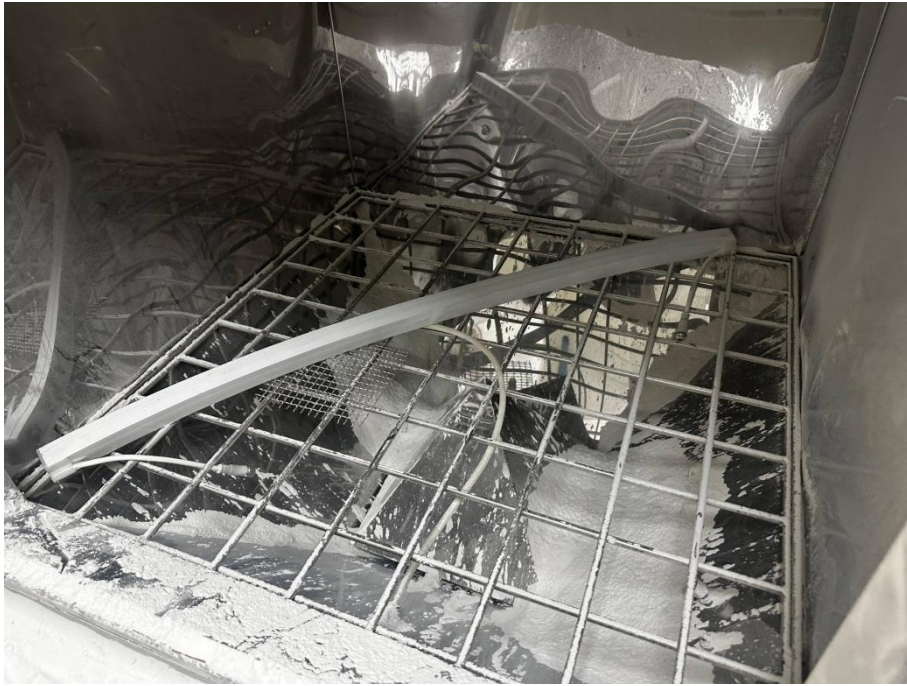
Photo 3: IP6X test of model FlexWash-06_3525-48
