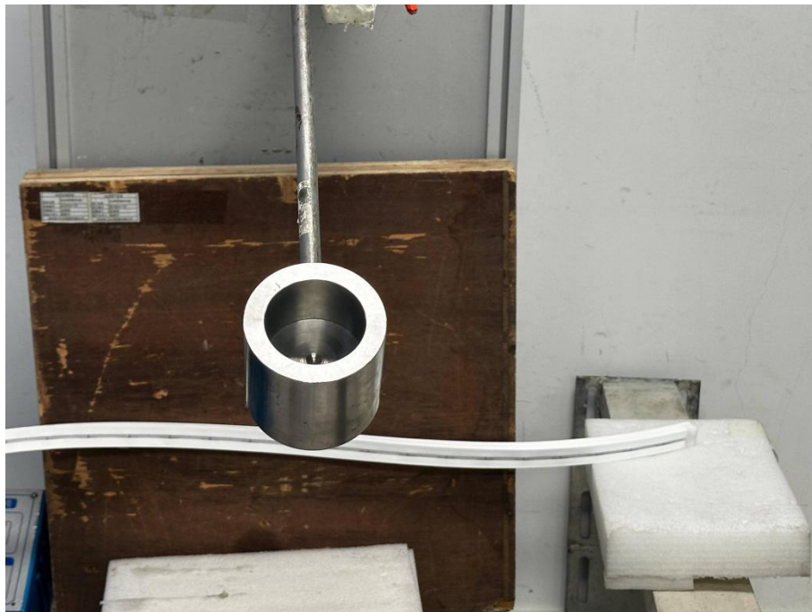
Photo 4: IK10 test of model NeonLine-01_2020-15
